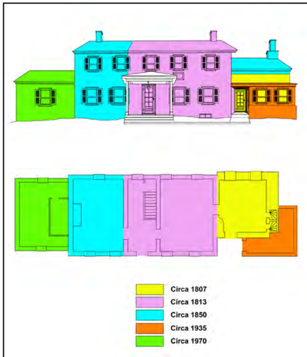
Figure 10 (left): Construction phases in the evolution of the stone farmhouse on the Joseph Lewis Farmstead are denoted on an elevation profile of the dwelling (top) and a footprint projection (bottom).
